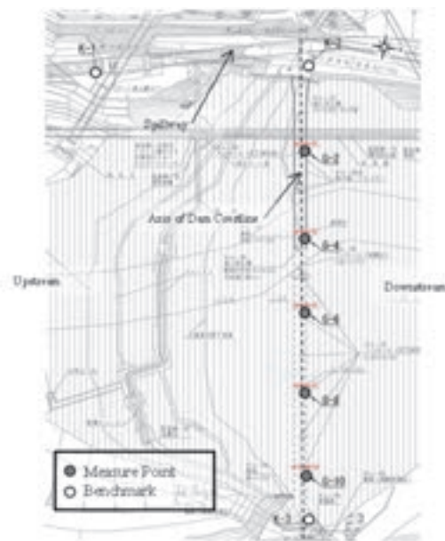
Figure 14. GPS Equipment Layout at Miboro dam
