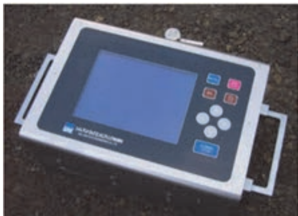
Figure 5. Portable RI meter, “WARP”
