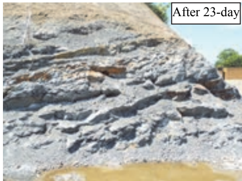
Figure 4. Slaking property of foundation rock after 23-day exposure
