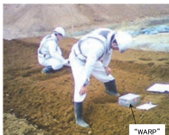
Figure 9. Measurement of water content by “WARP”
