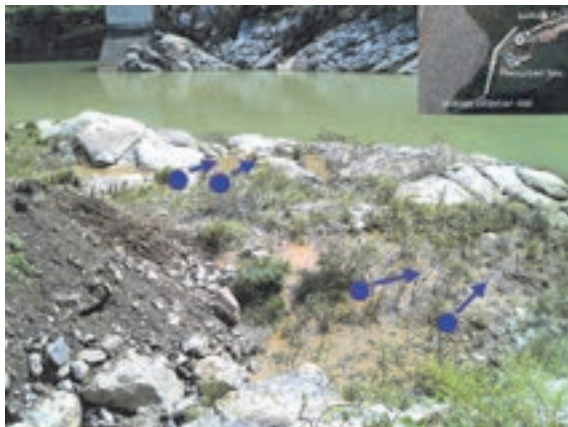
Figure 10. Flow out of pressurized water from the river bed
