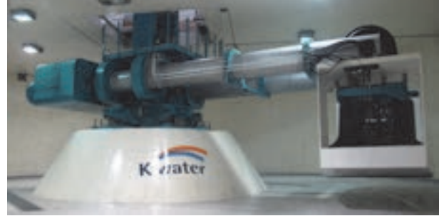
Figure 1. 800g-ton geotechnical centrifuge at K-water
