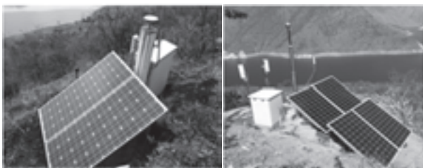
Figure 7. Standalone monitoring unit at a GNSS monitoring point for a slide body
