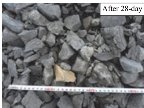
Figure 6. Slaking of CSG raw materials after 28-day exposure
