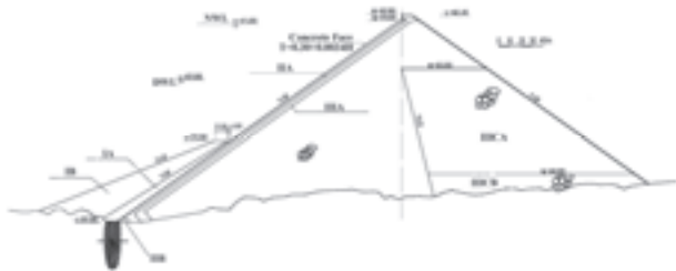
Figure 1. A typical cross section of Sanbanxi CFRD (HydroChina Zhongnan Engineering Corporation, 2008)
