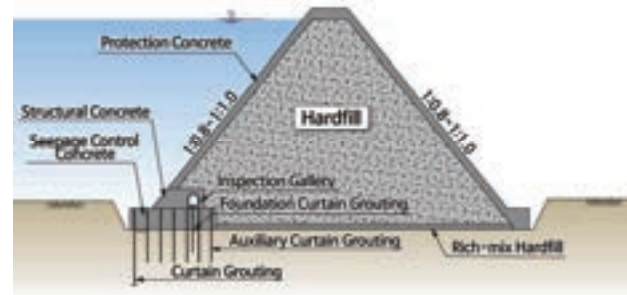
Figure 2. Schematic diagram for the Hardfill Dam method
