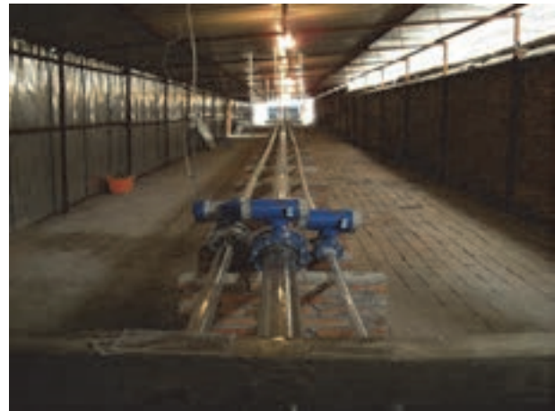
Figure 6 Resistance test in self-suction sediment transport piping model(1)
