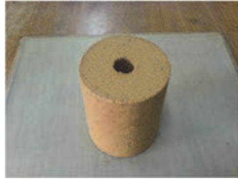
Figure 1. Soil specimen for hydraulic fracturing test
