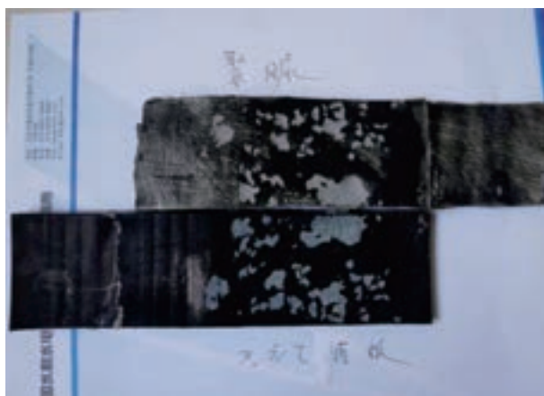
Figure.8 Surface Condition for peeling test of polyurea with PET nonwoven substrates coating- to-EPDM cover board
