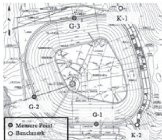
Figure 2. GPS Equipment Layout at Numappara dam
