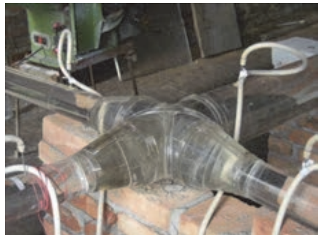
Figure 7 Resistance test in self-suction sediment transport piping model(2)
